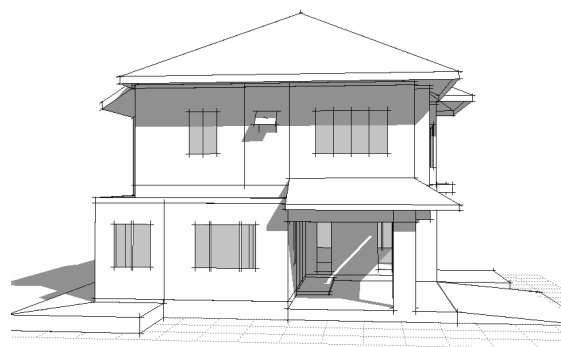
Figure 9: Inadequate shading on west façade of a contemporary house in the central region at 3pm in June (Source: Antarikananda, 2005)
