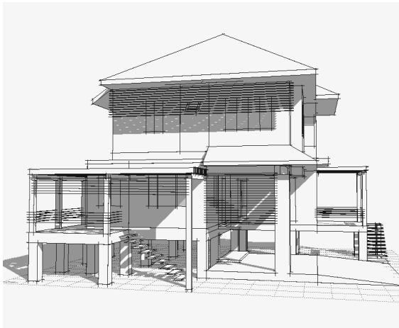
Figure 10: An improved contemporary design featuring additional shading, raised floors and shaded external platforms (Source: Antarikananda, 2005)
